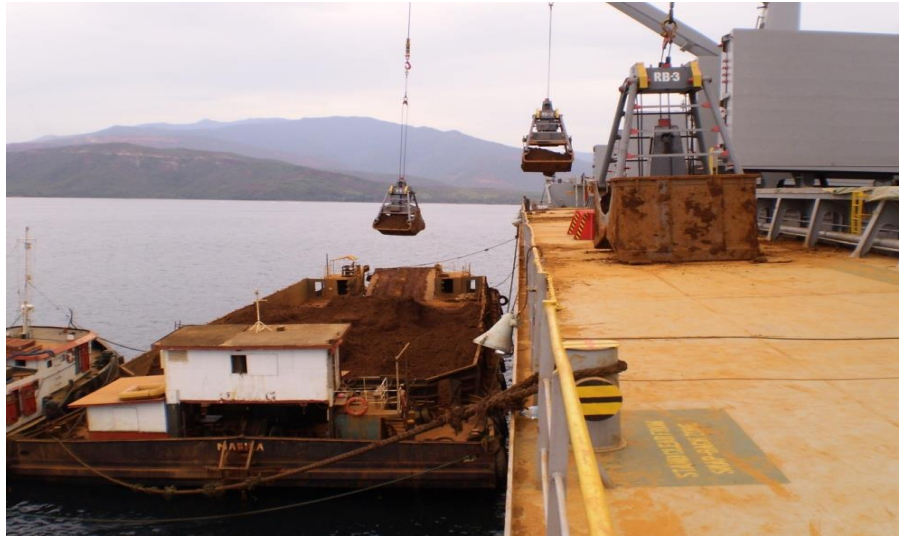
Figure 118. Loading of ore to vessel during shipment
