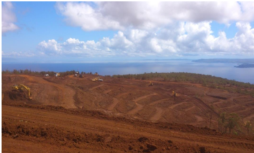
Figure 115. Bench forming and mining of ore
