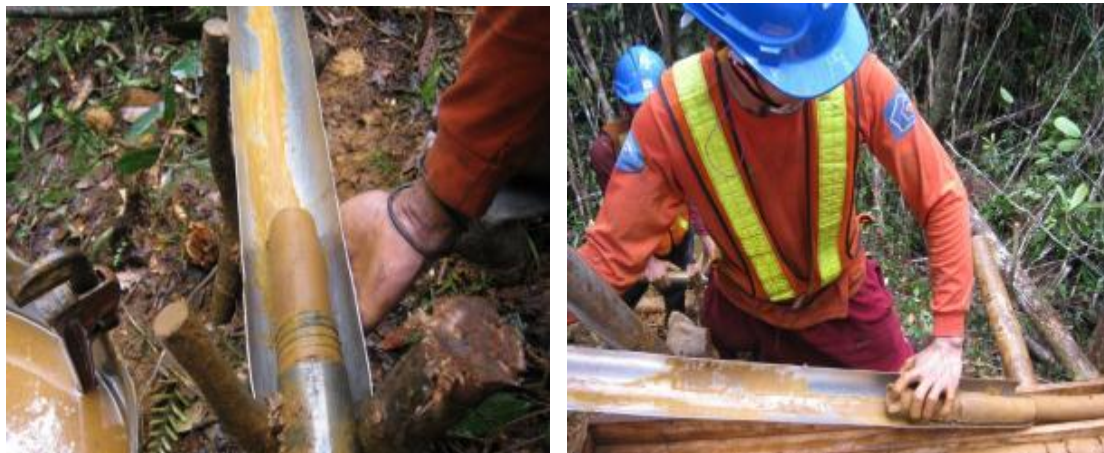
Figure-37. Core Extraction Prior to Core Logging/Sampling (Source: GPRI)
