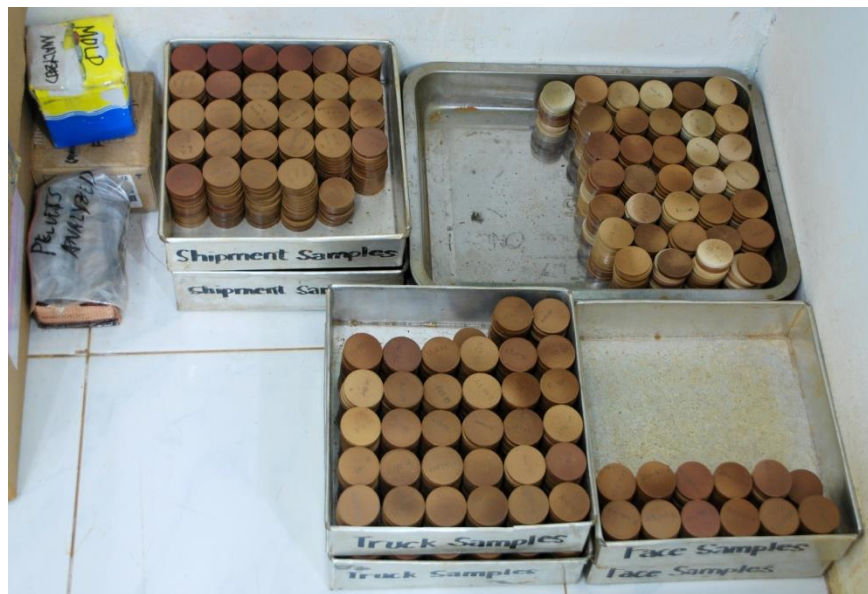
Figure-39. Pressed Pellets at PGMC Laboratory
