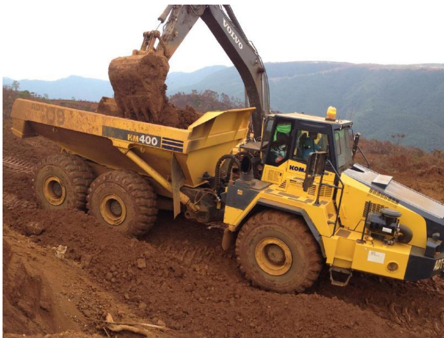
Figure-8: Excavator - Articulated Dump Truck Loading Operations (Source: Runge Pincock Minarco)
