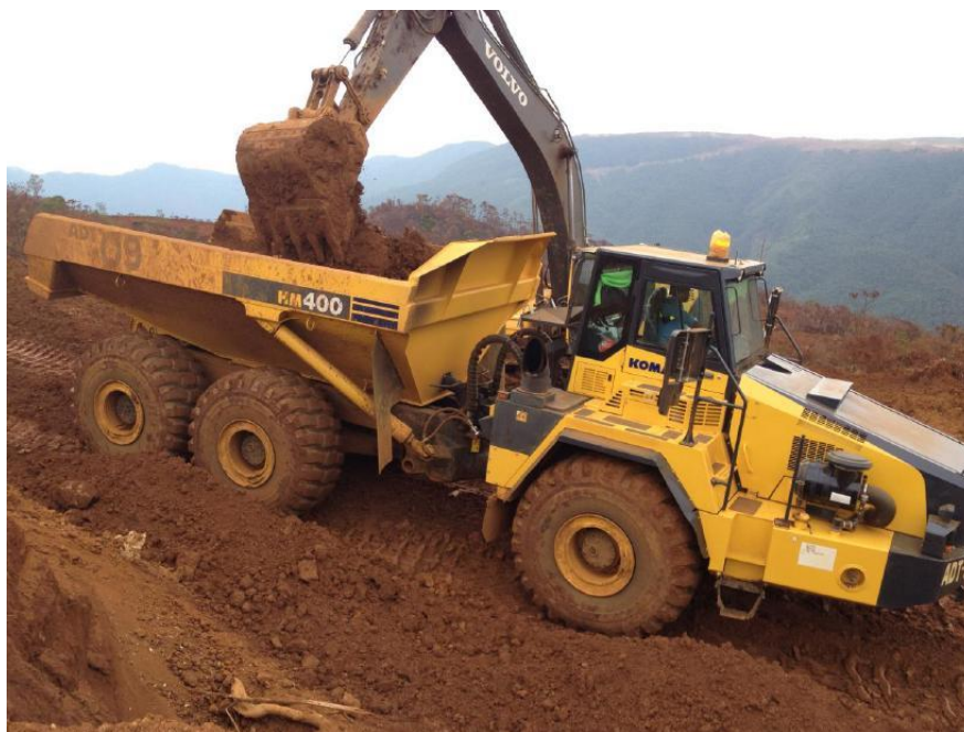
Figure-8: Excavator - Articulated Dump Truck Loading Operations (Source: Runge Pincock Minarco)
