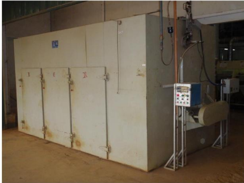
Figure-58. Thermostat-Controlled Manufactured Laboratory Oven at BNC Lab (Source: TMM)
