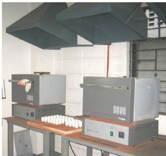
Figure-72. Barnstead Thermoline Furnace at ITS Manila (Source: TMM)
