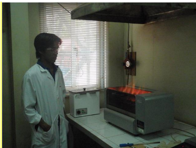
Figure-69. Sample Fusion using 6-place Claisse Fluxer at BNC Lab (Source: TMM)
