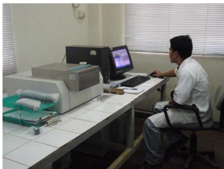
Figure-71. Spectro XEPOS Energy Dispersive X ray Fluorescence Instrument (Source: TMM)
