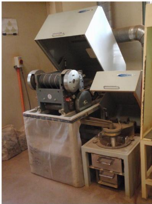
Figure-61. Rocklabs Boyd's Crusher w/ Automatic Splitter at BNC (Source: TMM)
