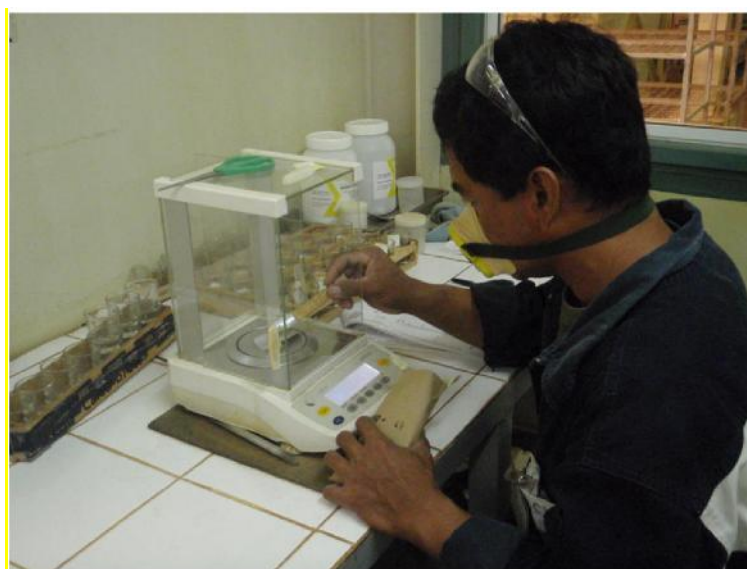
Figure-67. Microbalance Weighing of Pulverized Sample and Flux (Source: TMM)
