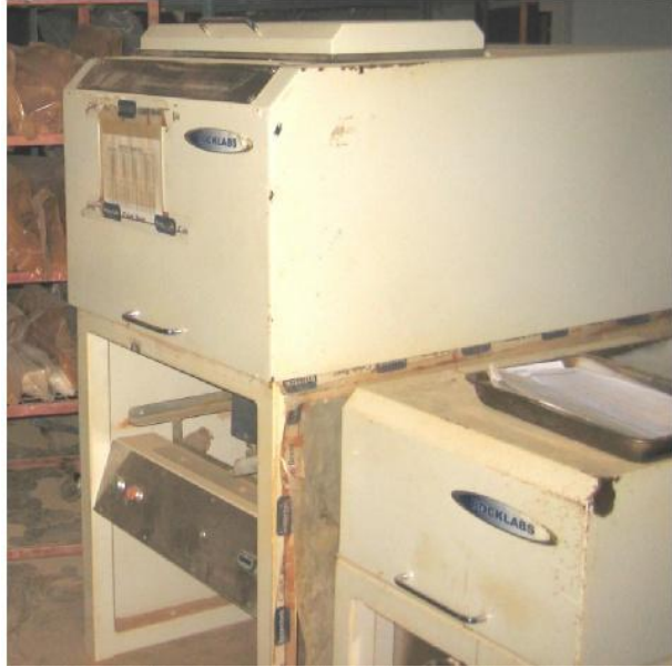
Figure-60. Rocklabs Boyd's Crusher with Automatic Splitter at ITS Manila (Source: TMM)
