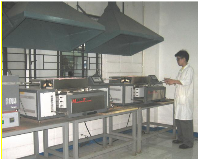
Figure-68. Sample Fusion using 6-place Modutemp Fluxer at ITS Manila (Source: TMM)
