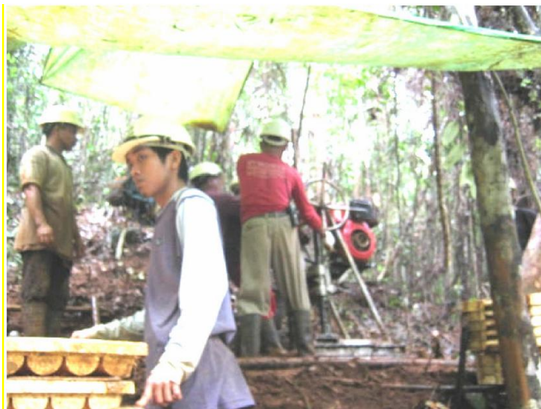
Figure- 47. Mechanical Portable Drill Rig in Operation (Source: TMM)
