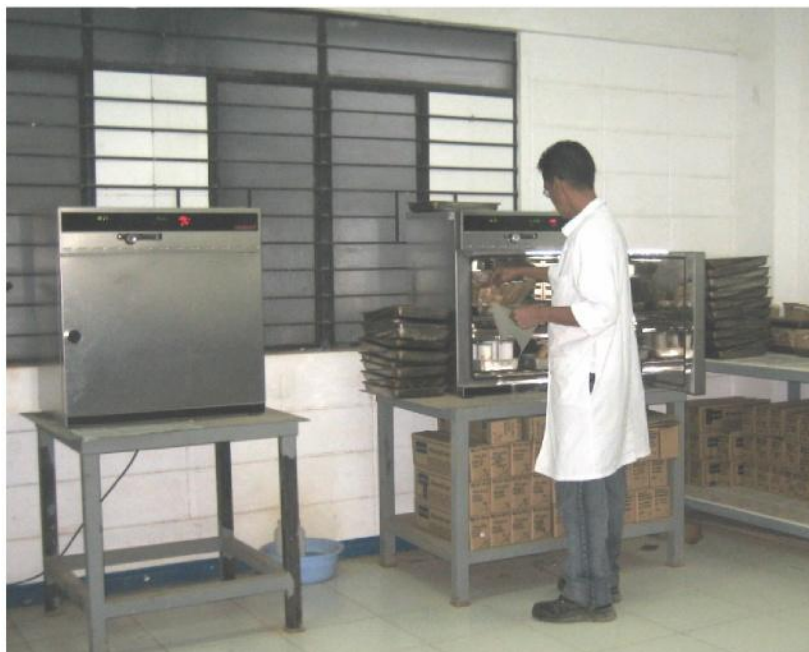
Figure-64. Pulverized Sample Drying with Memmert Electric Oven at ITS Manila (Source: TMM)
