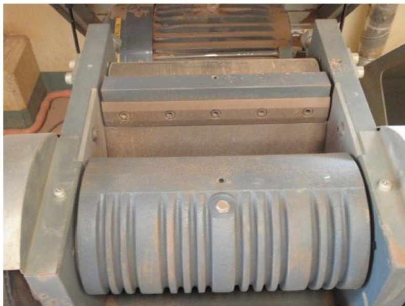
Figure-66. Jaw Plates of Crusher (Source: TMM)
